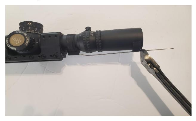
Step 6: You may need to add another slight bend to the rear of the wire to get the fiber housing to sit just right against the ocular or scope cap.
