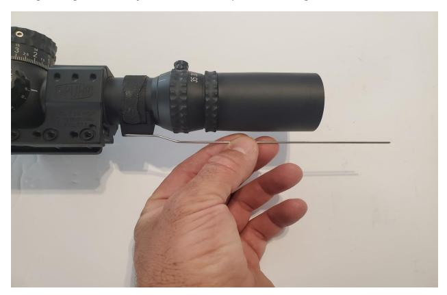
Step 5: Determine where the rear fiber housing will sit. This may vary if you're running a scope cap. Cut the stainless rod using dikes/ side cutters allowing the rod to fully insert into the housing.
