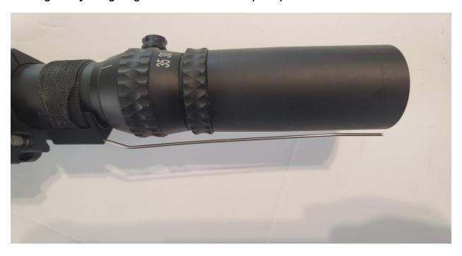
Step 8: Install the rear fiber housing onto the stainless rod using the smaller of the center most holes.
