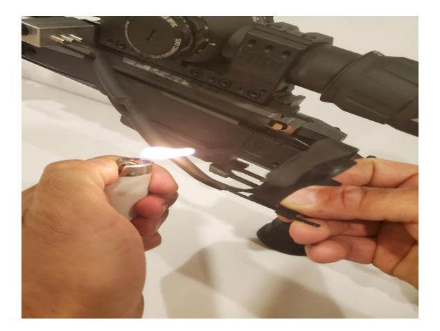
Step 12 Reinstall the leads on the gun and trim the leads about 1/16" past the ocular fiber rear housing, remove the fibers 1 more time from the rear housing, strip the outer housing back 1/8" and flame finish the ends same as you did in step 5. Reinstall the fibers into the rear housing making sure to insert them until the fiber is protruding past the back of the housing and you're done. (see pictures below)
