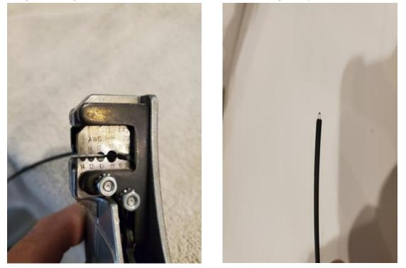
Step 8 Using a lighter flame finish the fiber on the stripped end of each of the 3 leads, hold the fiber near the side and base of the flame till you see the fiber start to ball up. The fiber only needs to be held close to flame, never contact the fiber to the flame and DONT over do it, the flame only needs to slightly
