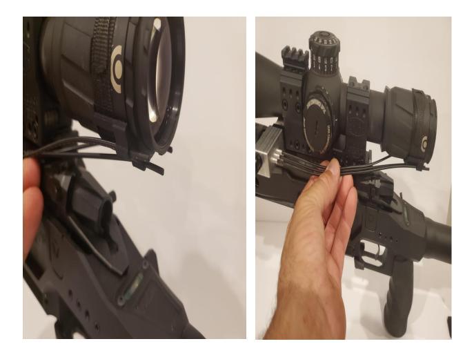
Step 10 determine the length of 1/2" heat shrink need to cover the main run of fiber bundle, measuring along the fiber bundle stopping and 5/8" short of either housing. Cut heat shrink to determined length, remove fibers from level housing and slide the heat shrink over the bundle then reinstall the ends into the housing and double checking you have reinstalled them in the appropriate locations. (see picture below)
